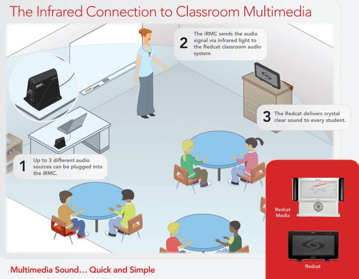
The iRMC can be placed near classroom audio sources for a quick connect solution. Running wires and cables around the room is no longer necessary. Whatever multimedia sound source you choose will be heard clearly throughout the learning environment.
