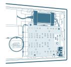
Close the speaker door and slide it toward the middle of Topcat to lock it into place.
